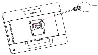
6).Remove the extended interface cover: pull the expanded interface cover outward at the notch according to the picture shows, and remove it.
