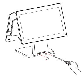
**2).**After removing the screw, pull at the back shell of the base according to the picture shows, and remove the back shell of the base.
