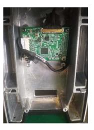
3).Remove the two connectors shown in the picture and protect them with the tape according to the picture shows
