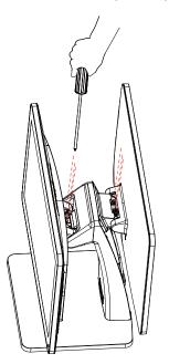
5).Remove the hinges of the host: Remove four screws according to the picture shows. Remove the hinges of the host and the hinges cover of the host separately.
