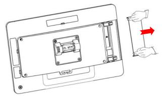
7. remove the hard drive, unscrew the hard drive fixing screw, then remove the hard drive as arrow
