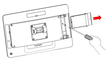
8.remove the host back cover, remove the screws of hinge cover(4 pcs, show as ①) and screws of back cover(4 pcs, show as ②), then remove the back cover ,and then you may replace or maintenance the mainboard.
