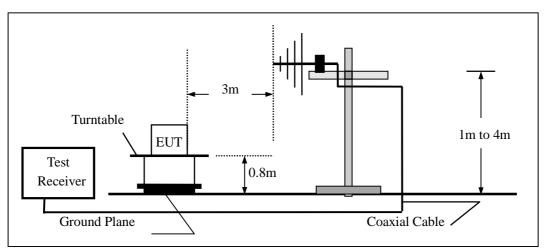
(c) For radiated emissions above 1000MHz
