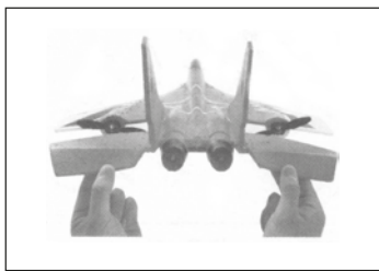
IF THE ASCENDING ANGLE IS TOO BIG WHEN TAKING OFF, YOU CAN TRIM THE LEVEL TAIL WING DOWNWARD.
