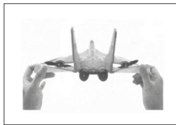
IF THE AIRPLANE CAN NOT RISE UP ITS NOSE WHEN TAKING OFF, YOU CAN TRIM THE LEVEL TAIL WING UPWARD.
