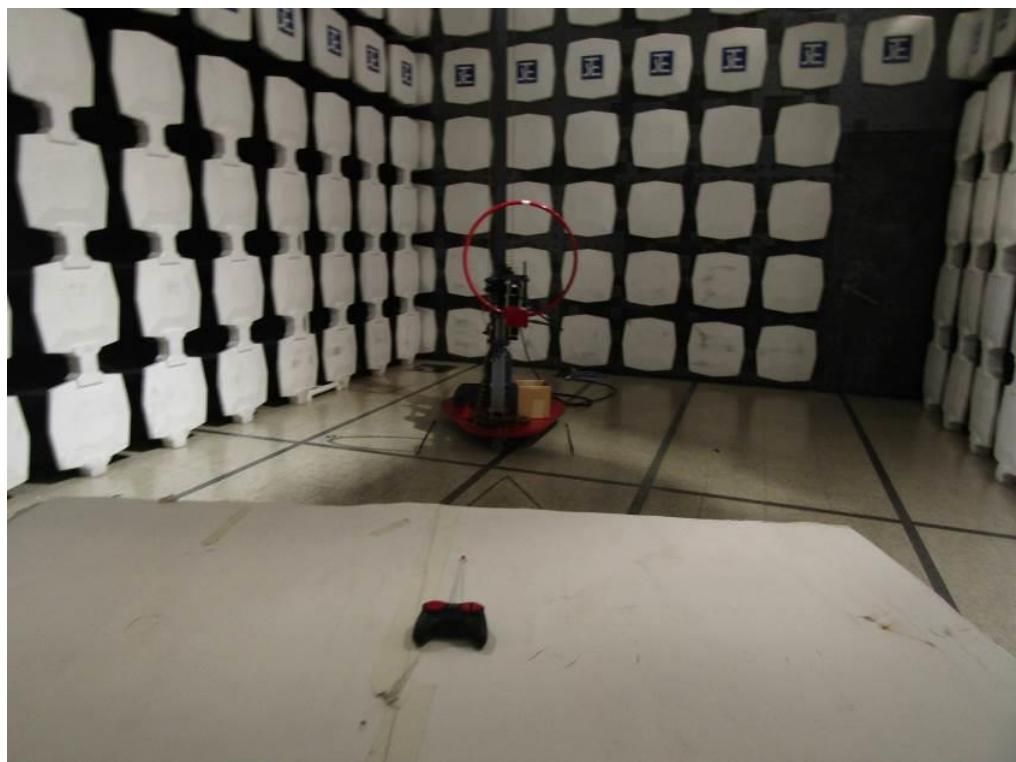
**Measurement of Radiated Emission Test Set Up (30-1000MHz)**
