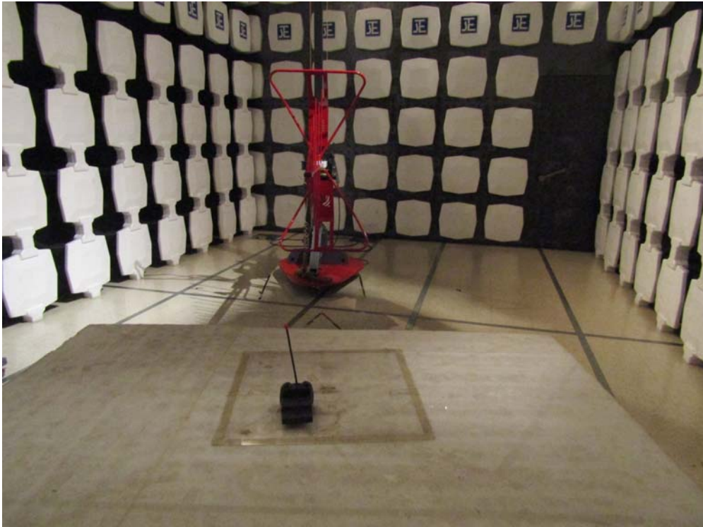
Measurement of Radiated Emission Test Set Up
