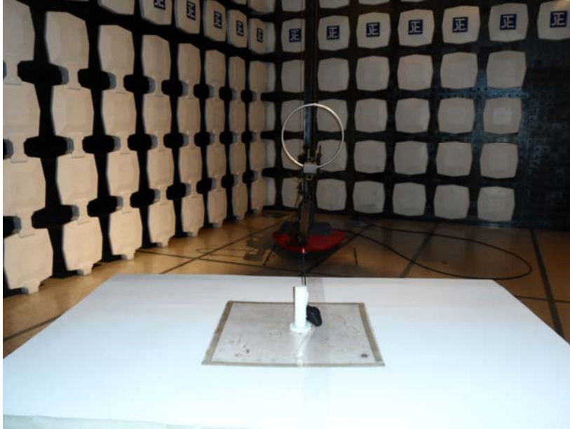
Measurement of Radiated Emission Test Set Up
