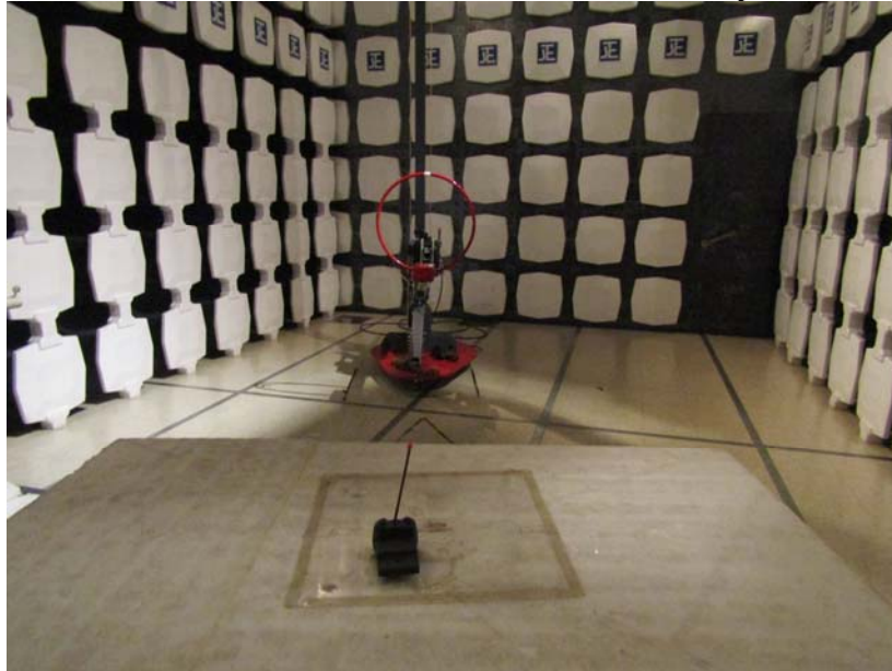
Measurement of Radiated Emission Test Set Up
