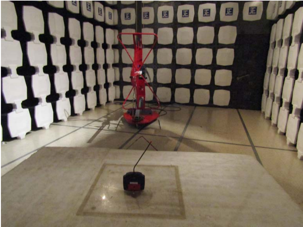
Measurement of Radiated Emission Test Set Up
