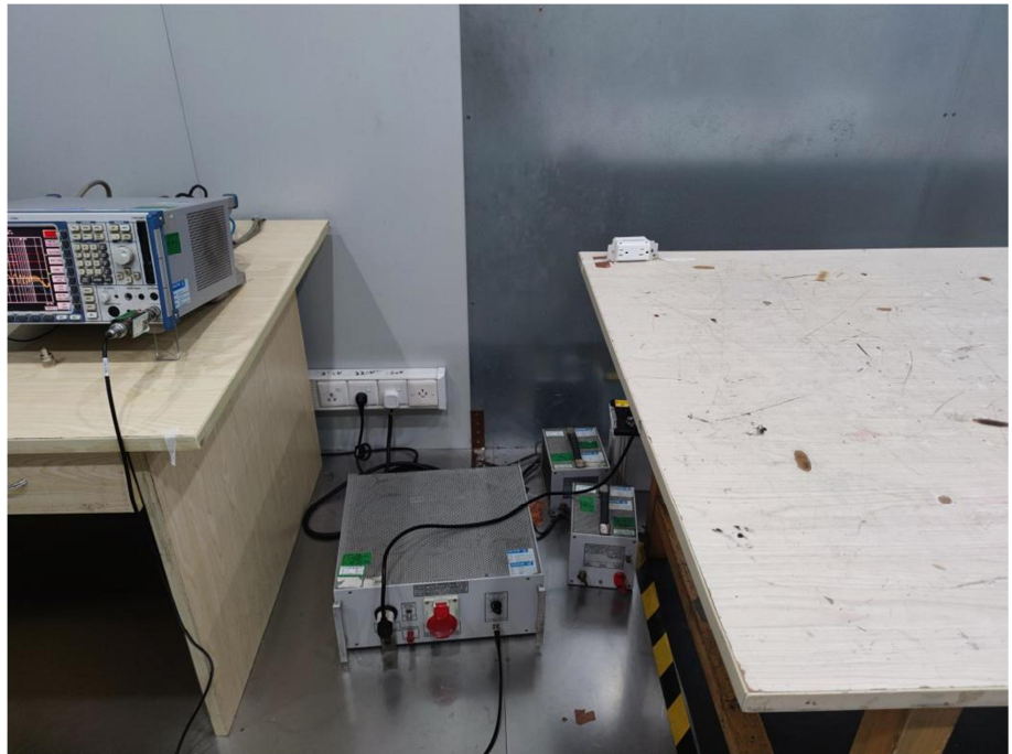
Conducted Emission Test Setup
