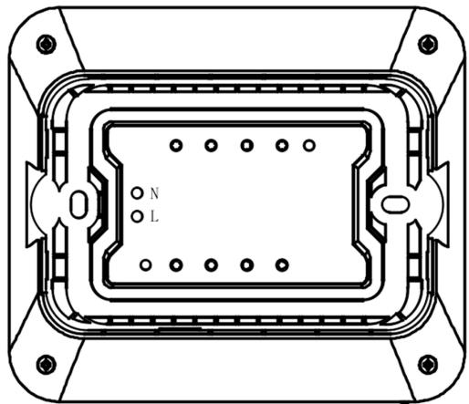
4. Fix the bottom case on the interior wall cassette with screws, pay attention to the mounting direction
