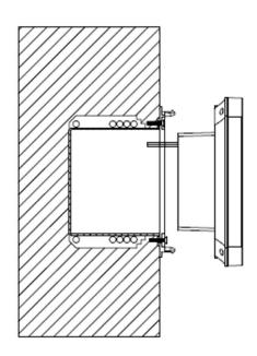
6. Press the lower end of the panel to the bottom case to complete the product installation
