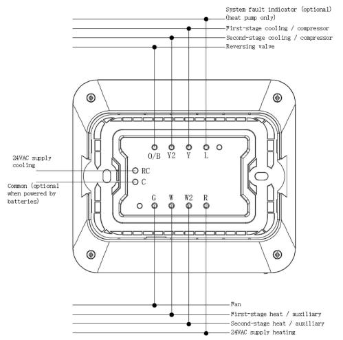
4. Fix the bottom case on the interior wall cassette with screws, pay attention to the mounting direction
