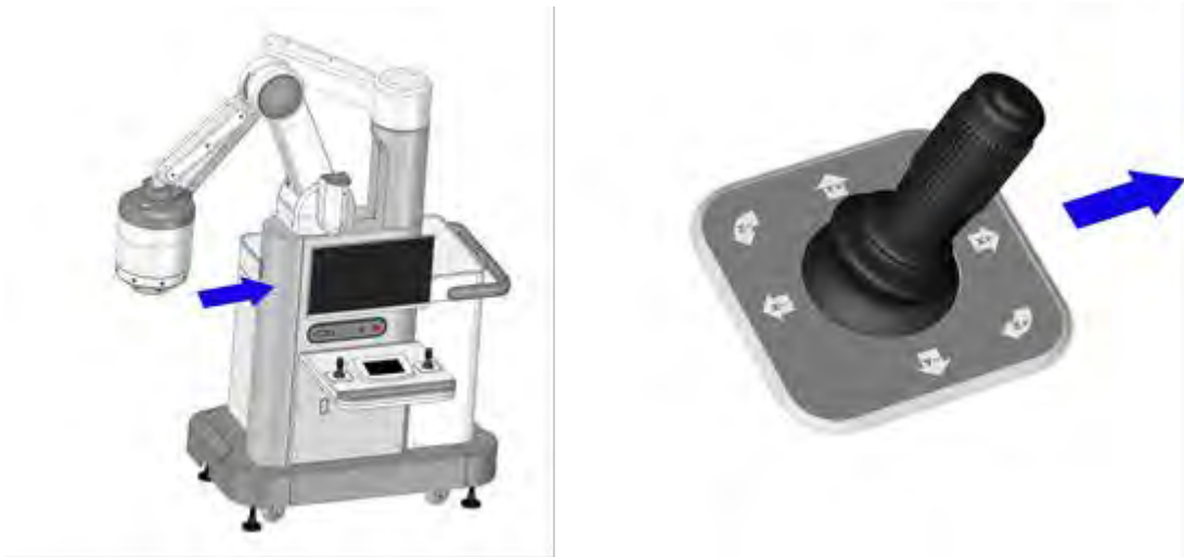
Figure 3-9 :Move in direction along X+ axis
