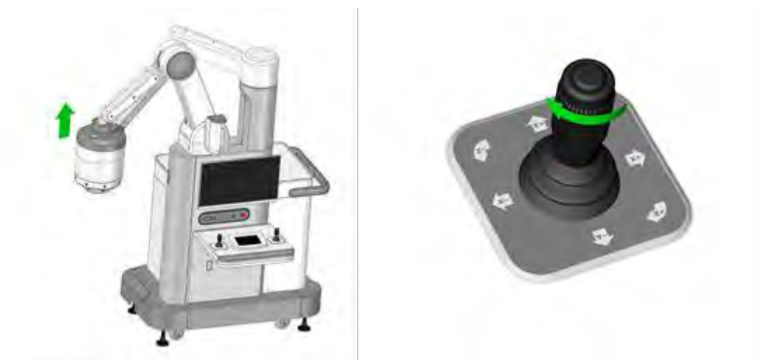
Figure 3-13: Move in direction along Z+ axis
