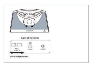
To conserve battery power, the Receiver will turn itself off if no audio signal is received from the base transmitter for a period longer than 5 minutes, (example, the TV is turned off). The volume knob ring light will be off.
