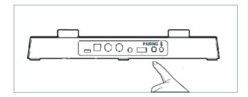
3. Press and hold the PAIRING button on the side of the new Receiver until the volume knob ring indicator starts blinking.
