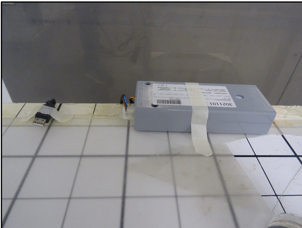
Photo 12 AC Conducted Emissions Test Setup
