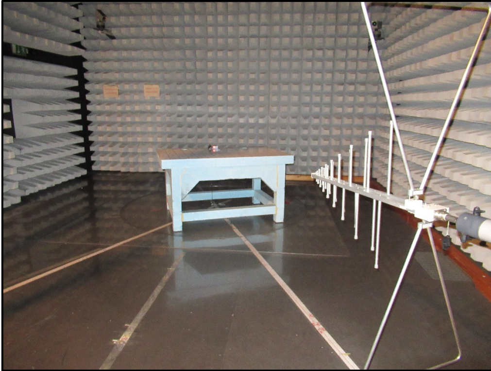
Photo 3: Radiated Test Setup-30 MHz to 1GHz
