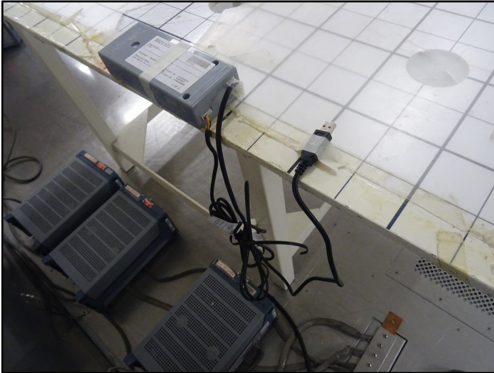
Photo 11 AC Conducted Emissions Test Setup
