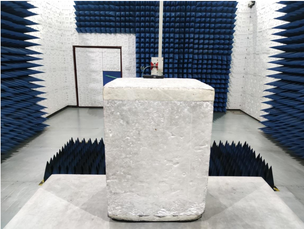
RADIATED EMISSION TEST SETUP ABOVE 1GHz
