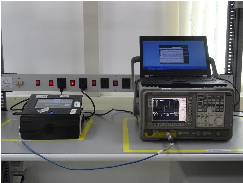
Antenna Port measurement Setup
