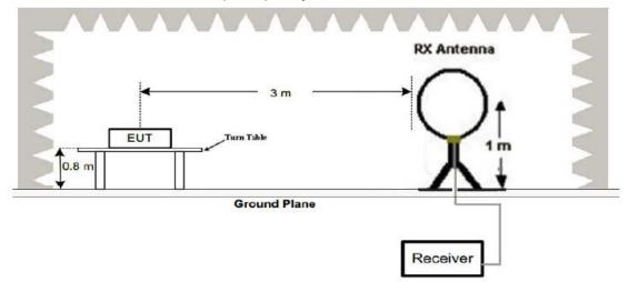
(2) Radiated Emission Test-Up Frequency 30MHz~1GHz
