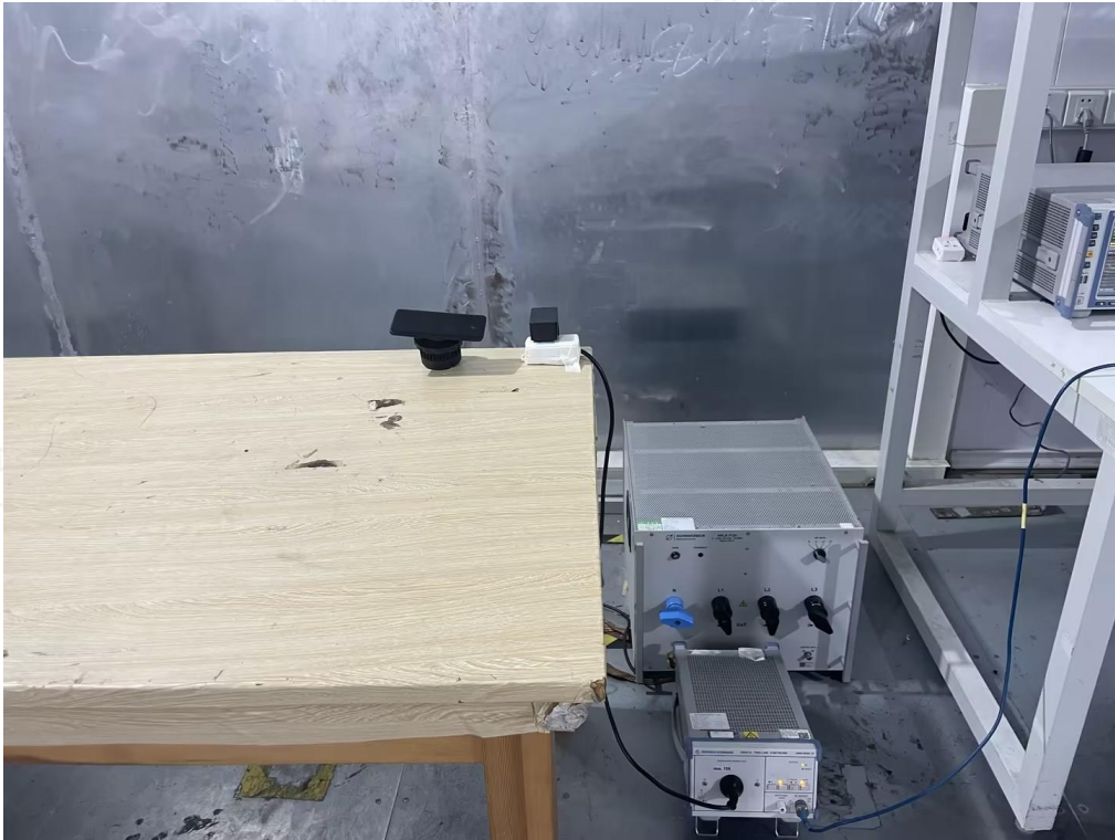
Conducted Emission-AC adapter charge mode
