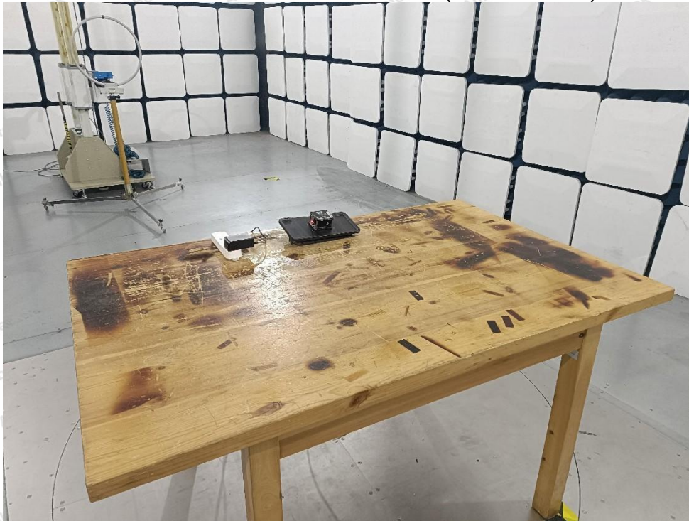
Photo of Radiation Emission Test (below 30MHz)
