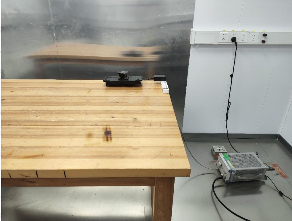
Photo of Conducted Emission Measurement
