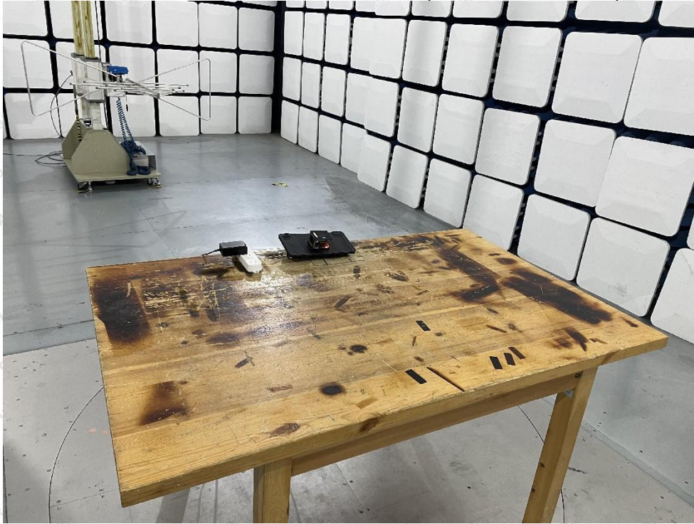
Photo of Radiation Emission Test (30MHz~1000MHz)
