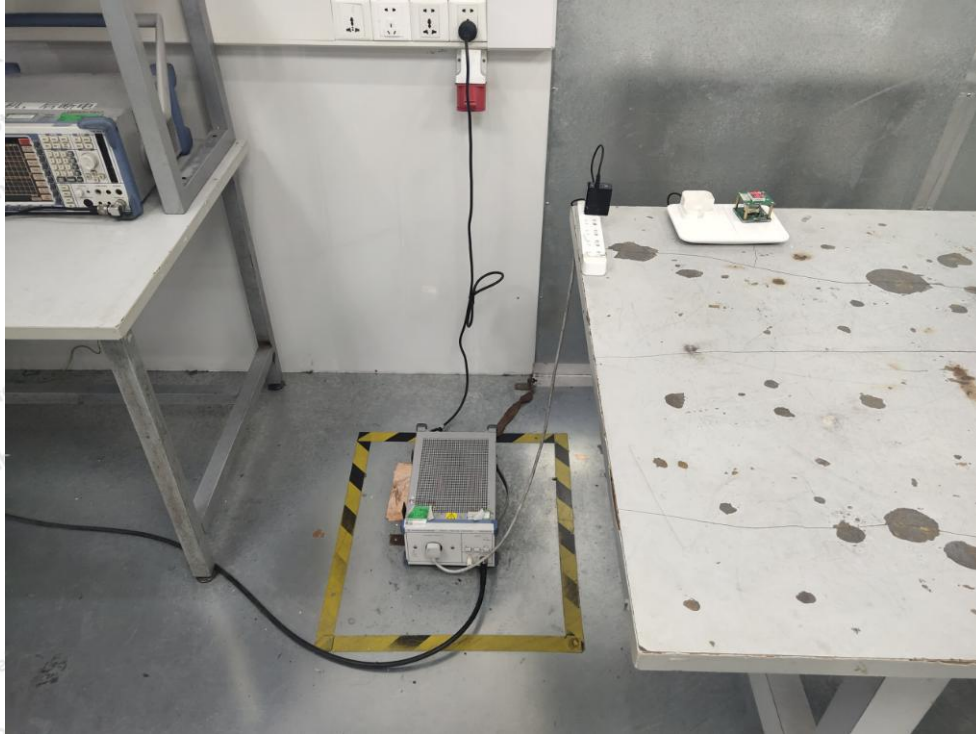
Photo of Conducted Emission Measurement
