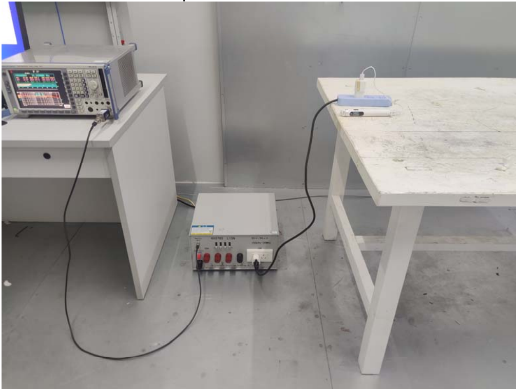
Photos of power line conducted emission test
