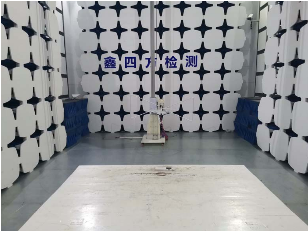
Photos of radiated emission test 30MHz – 1GHz
