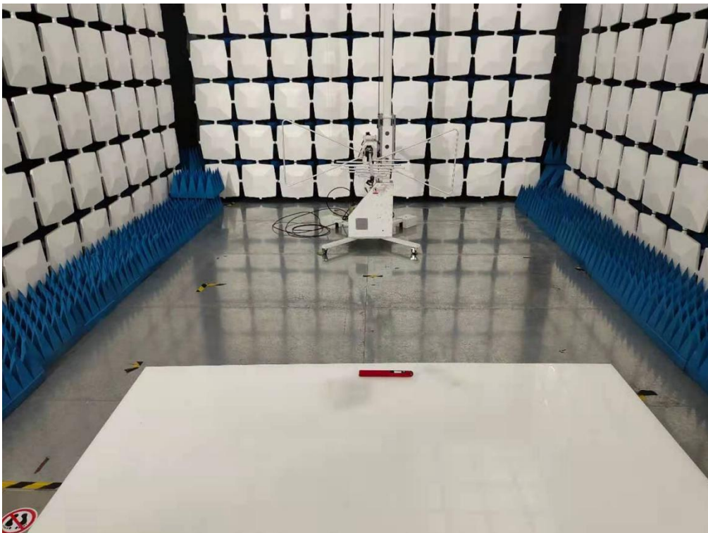
Below 1GHz for radiated emission test setup
