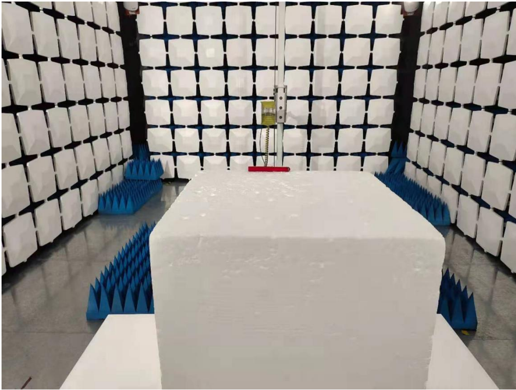
Above 1GHz for radiated emission test setup
