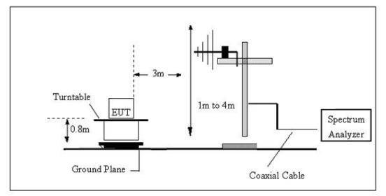
(C) Radiated Emission Test-Up Frequency Above 1GHz
