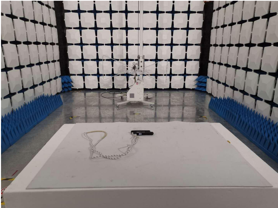
Below 1GHz for radiated emission test setup
