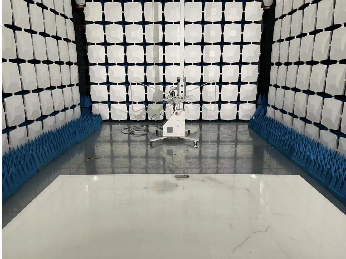
Above 1GHz for radiated emission test setup
