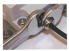
The tightening torque is 6 Nm. You can check this with the help of a suitable torque wrench to be certain:
