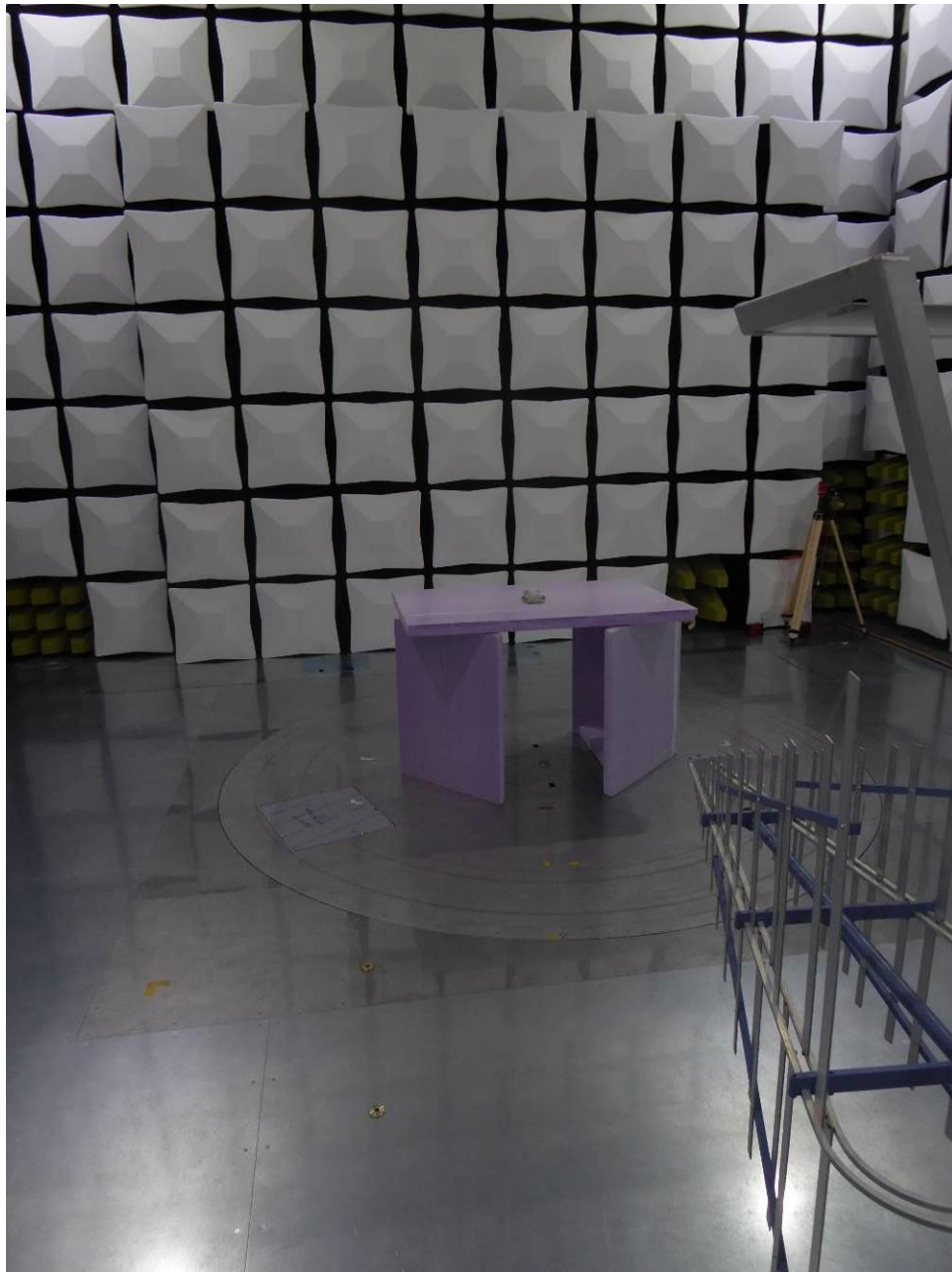
Test setup – radiated test in semi-anechoic chamber Preliminary measurement 30 – 1000 MHz
