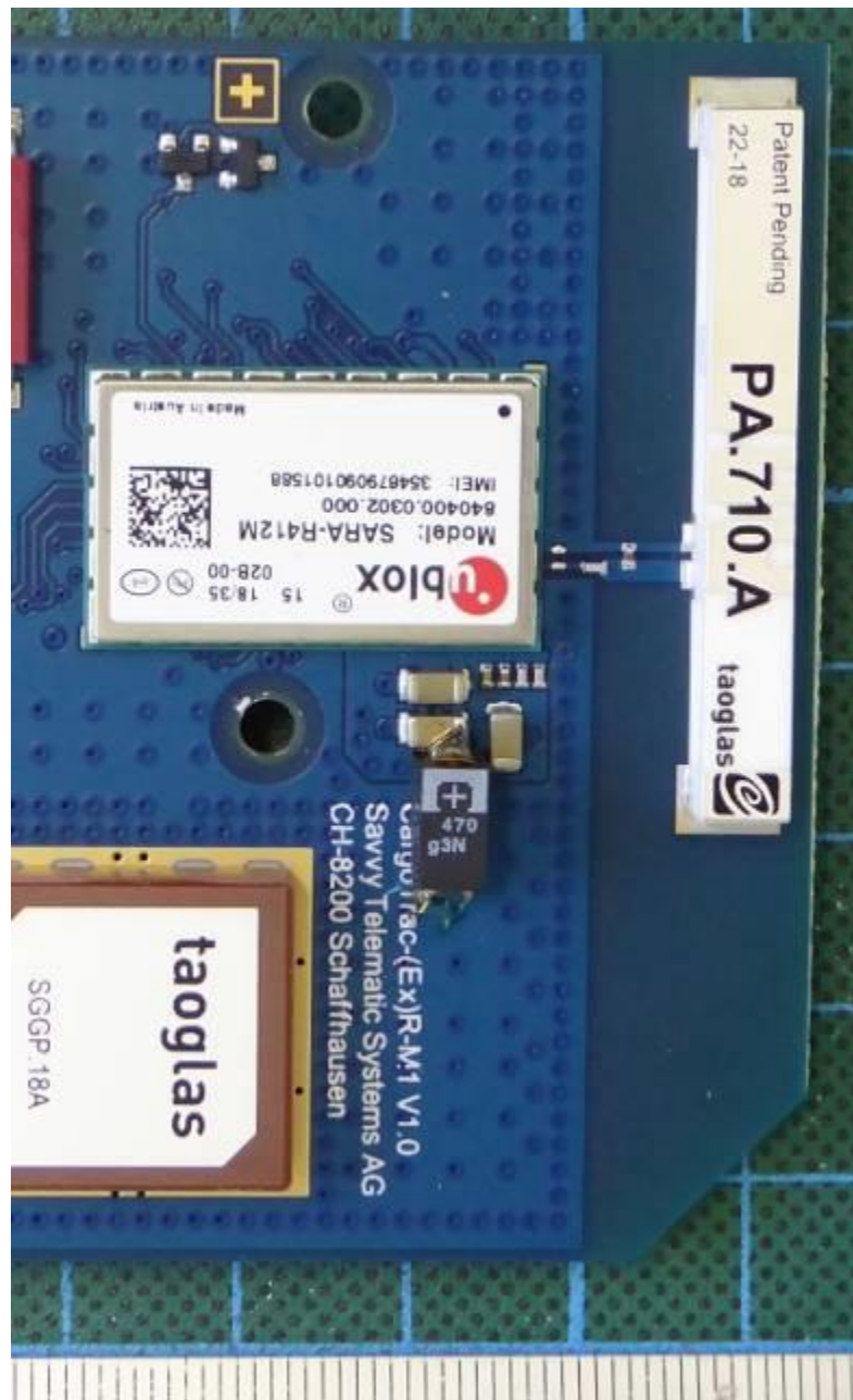
EUT cellular radio module and antenna Detail view
