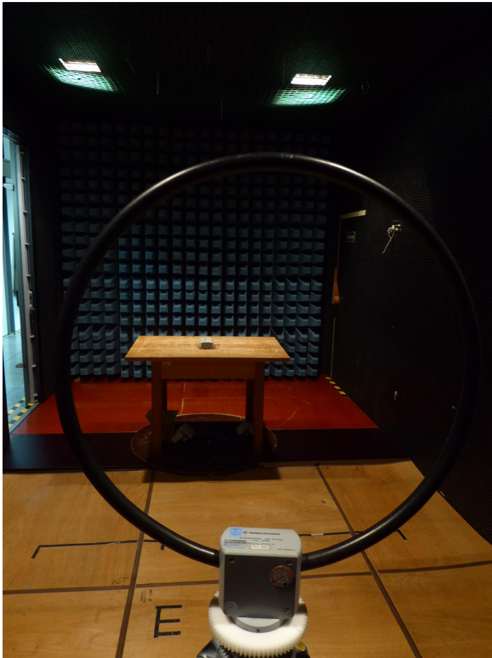
Test setup – radiated test in anechoic chamber Preliminary measurement 9 kHz - 30 MHz
