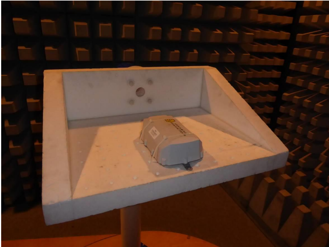
Test setup – radiated test in anechoic chamber
