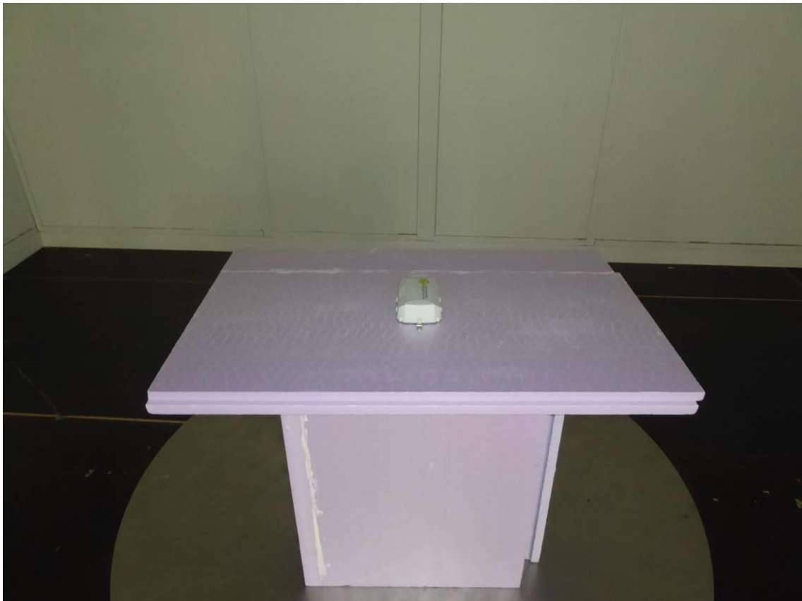
Test setup – radiated test on open area test site Final measurement 30 – 1000 MHz
