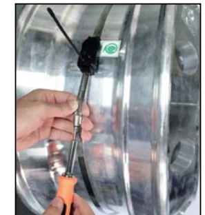
③ Pre tighten steel tie screw
