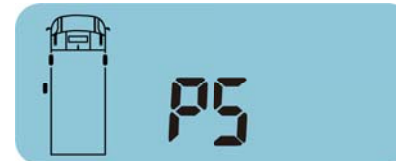
( figure 3 : Rear Left outer tire blinks,press" SET" key to switc )
