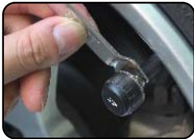
Reverse fixed sensors and screw
