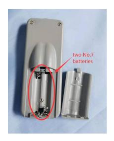
The main components of the exciter are single chip microcomputer, battery, 125kHz low frequency antenna and two No. 7 batteries. There are 6 buttons and 1 red indicator light on the surface of the activator. Long press any key to send 125kHz low frequency signal, which can wake up the sensor within 20cm distance. When the sensor receives the low frequency signal, it will immediately transmit the data signal. Users can read sensor information through TPMS display.
