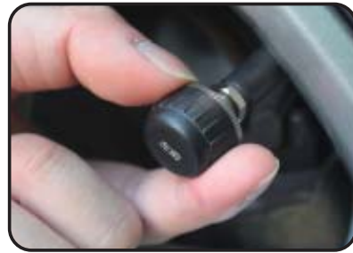
Installation the sensor
