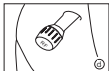
Ensure the external sensor is tightened properly and check for any possible air leakage before using it.
