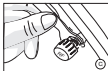
Tighten to lock the external sensor using the spanner (provided) onto the valve.
