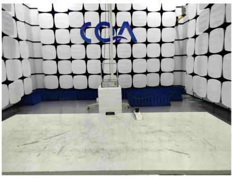
Radiated emission Test Setup-2 (30MHz~1GHz)
