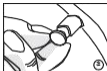
Remove the original valve cover and install the anti-theft screw on the valve.
