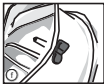
TPMS device installation completed. continue by fitting the tyre back onto the wheel.
