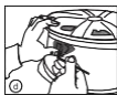
Install & adjust TPMS sensor unit (adjustable) onto wheel to sit flush onto the wheel barrel.
