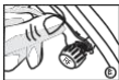
Tighten to lock the external sensor using the spinner (provided) onto the valve.
