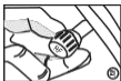
Install the external TPMS sensor on the existing valve according to the dedicated location on each side of the vehicle.
