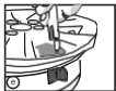
Install the front side TPMS valve by screwing and tighten the valve socket on the face of wheel.
