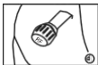
Ensure the external sensor is tightened properly and check for any possible air leakage before using it.
