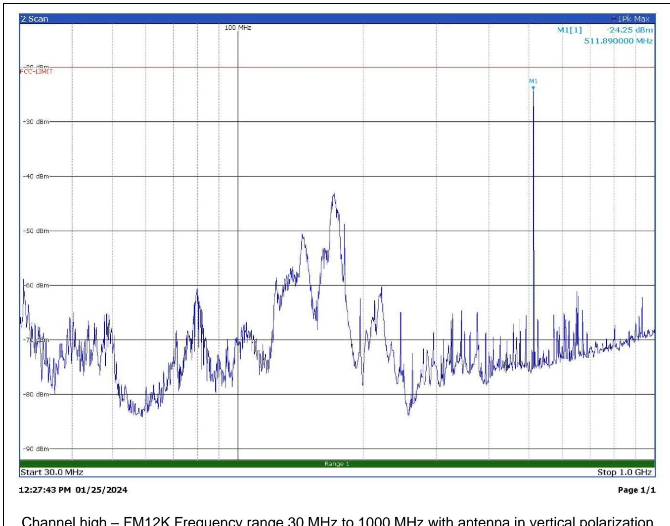
Channel high – FM12K Frequency range 30 MHz to 1000 MHz with antenna in vertical polarization
