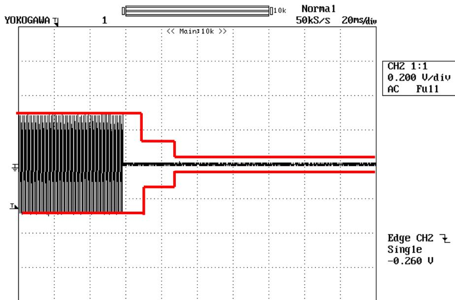
Switch on condition,  $t_1=10$  ms,  $t_2=25$  ms, 481 MHz, channel separation  $\pm 12.5$  kHz
