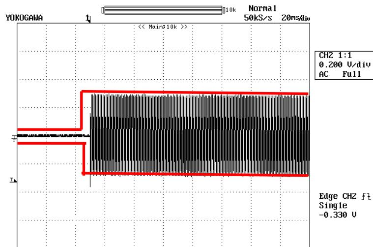
Switch off condition,  $t_3=10$  ms, 481 MHz, channel separation  $\pm 12.5$  kHz
