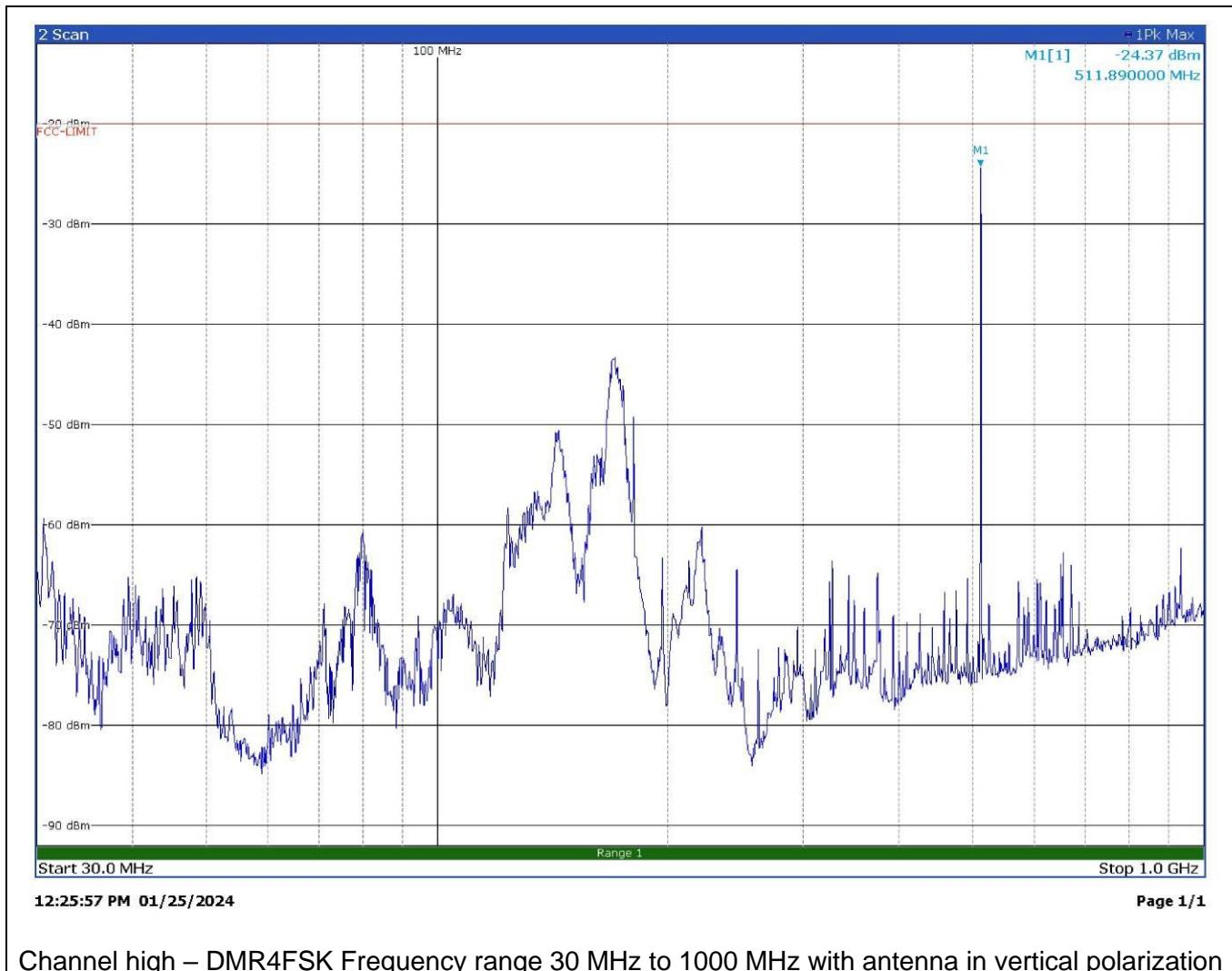
Channel high – DMR4FSK Frequency range 30 MHz to 1000 MHz with antenna in vertical polarization
