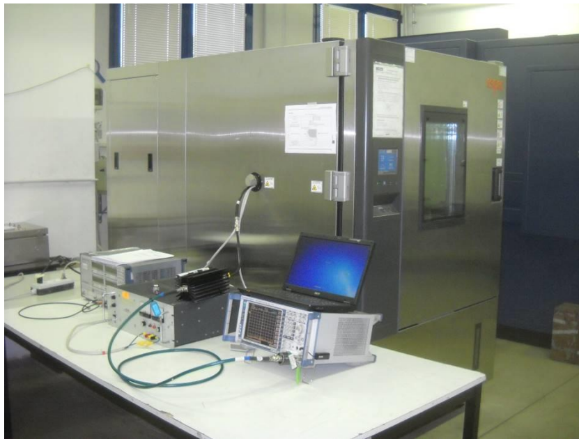
Set-up photo for frequency error tests
