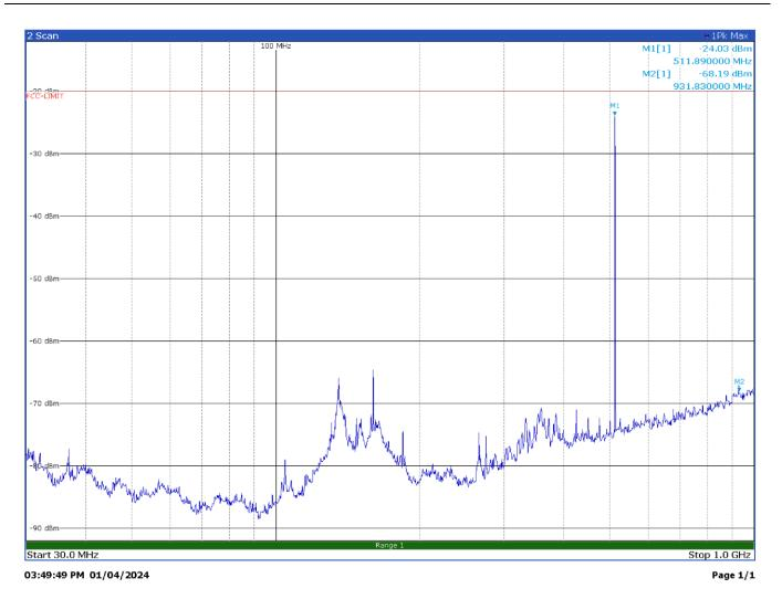
Radiated spurious emissions with modulation FM 12.5 kHz at 511.9 MHz – Antenna in horizontal polarization
