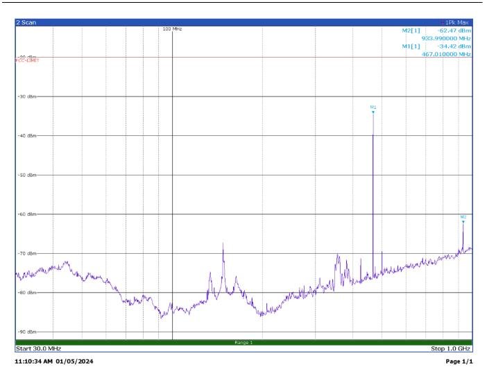
Radiated spurious emissions with modulation CST 4FSK at 467.0 MHz – Antenna in horizontal polarization
