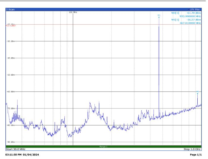
Radiated spurious emissions with modulation DMR 4FSK at 467 MHz – Antenna in vertical polarization
