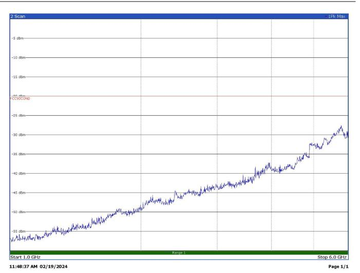
Radiated spurious emissions with modulation CST 4FSK at 420.1 MHz – Antenna in horizontal polarization
