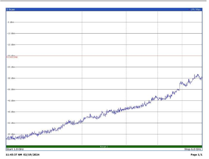
Radiated spurious emissions with modulation FM 12.5 kHz at 420.1 MHz – Antenna in vertical polarization
