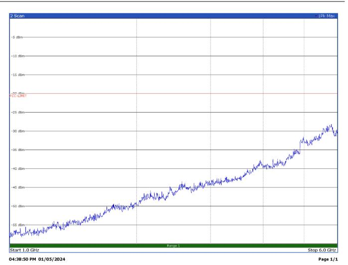
Radiated spurious emissions with modulation FM 25.0 kHz at 467 MHz – Antenna in horizontal polarization
