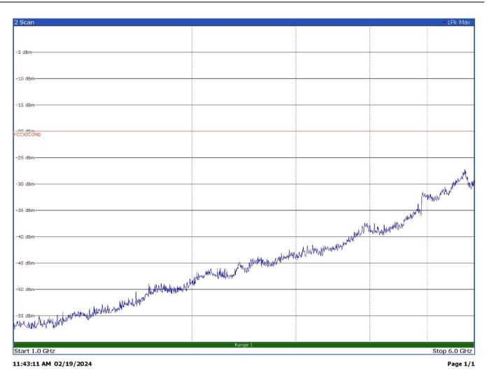
Radiated spurious emissions with modulation DMR 4FSK at 420.1 MHz – Antenna in vertical polarization
