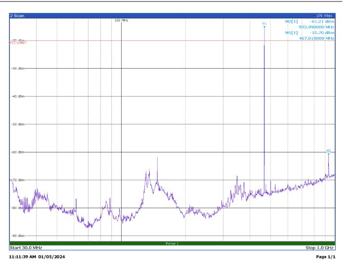
Radiated spurious emissions with modulation CST 4FSK at 467.0 MHz – Antenna in vertical polarization
