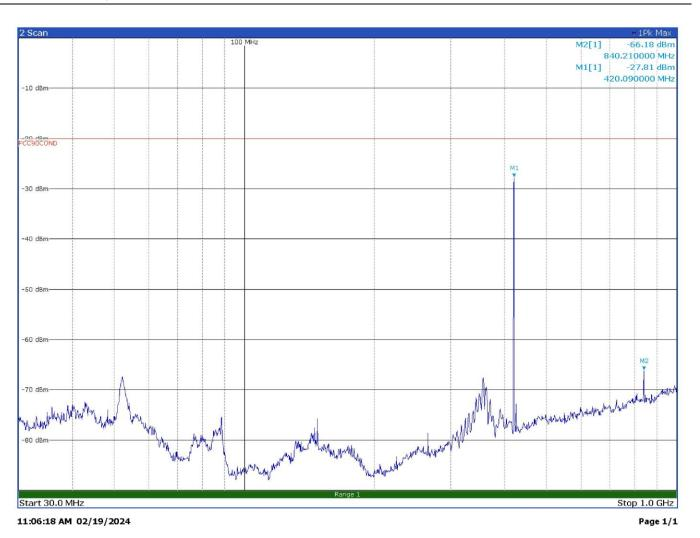
Radiated spurious emissions with modulation FM 12.5 kHz at 420.1 MHz – Antenna in horizontal polarization
