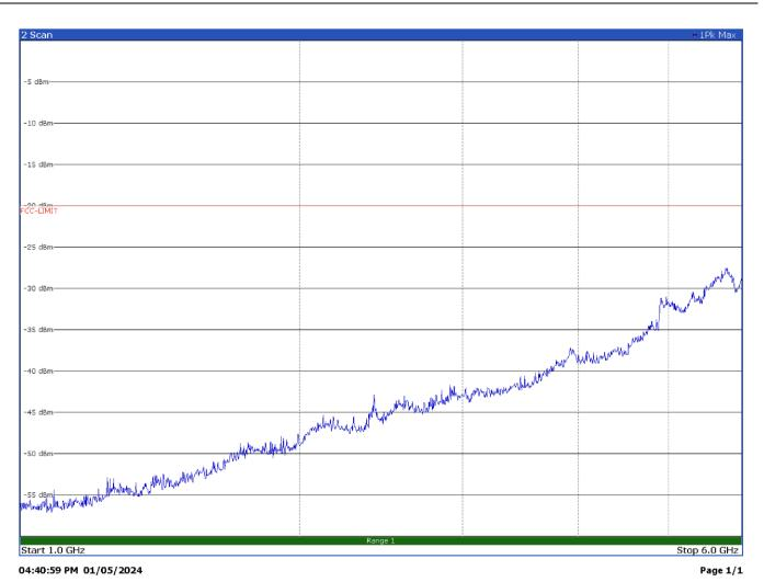
Radiated spurious emissions with modulation FM 25.0 kHz at 511.9 MHz – Antenna in vertical polarization
