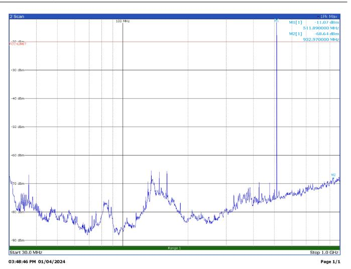
Radiated spurious emissions with modulation FM 12.5 kHz at 511.9 MHz – Antenna in vertical polarization
