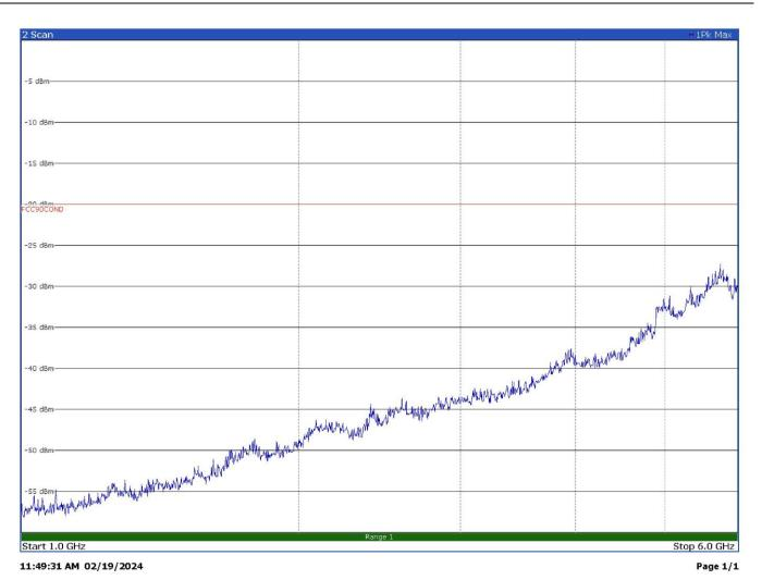
Radiated spurious emissions with modulation CST 4FSK at 420.1 MHz – Antenna in vertical polarization
