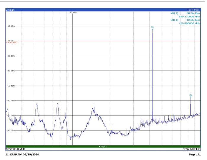
Radiated spurious emissions with modulation FM 25.0 kHz at 420.1 MHz – Antenna in vertical polarization
