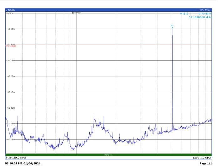
Radiated spurious emissions with modulation DMR 4FSK at 511.9 MHz – Antenna in vertical polarization
