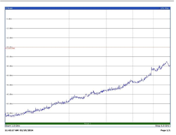
Radiated spurious emissions with modulation DMR 4FSK at 420.1 MHz – Antenna in horizontal polarization
