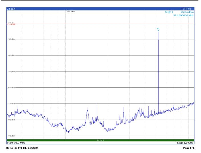
Radiated spurious emissions with modulation DMR 4FSK at 511.9 MHz – Antenna in horizontal polarization
