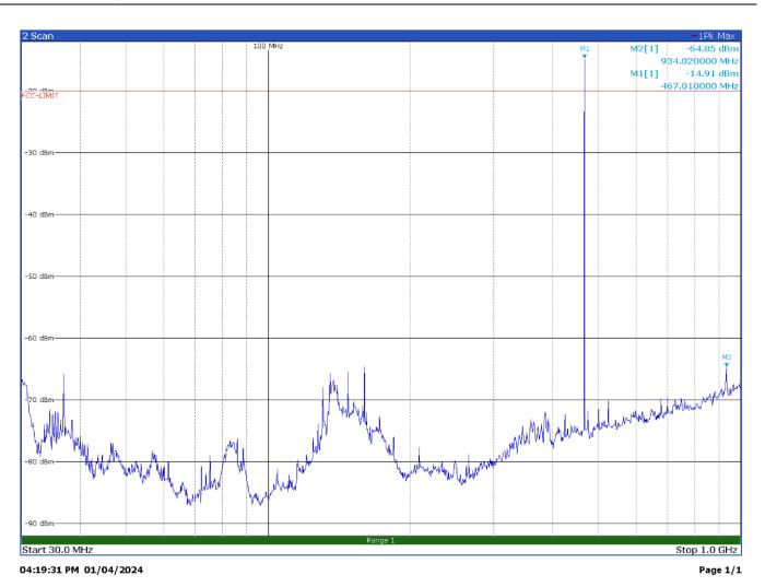
Radiated spurious emissions with modulation FM 25.0 kHz at 467 MHz – Antenna in vertical polarization
