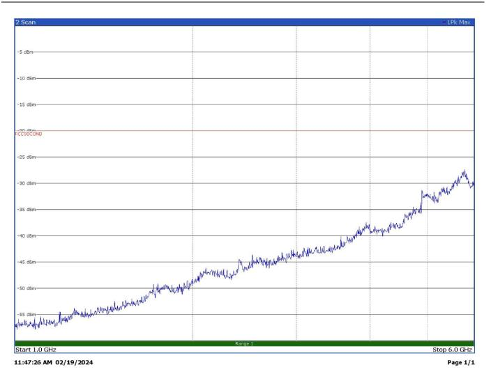
Radiated spurious emissions with modulation FM 25.0 kHz at 420.1 MHz – Antenna in horizontal polarization
