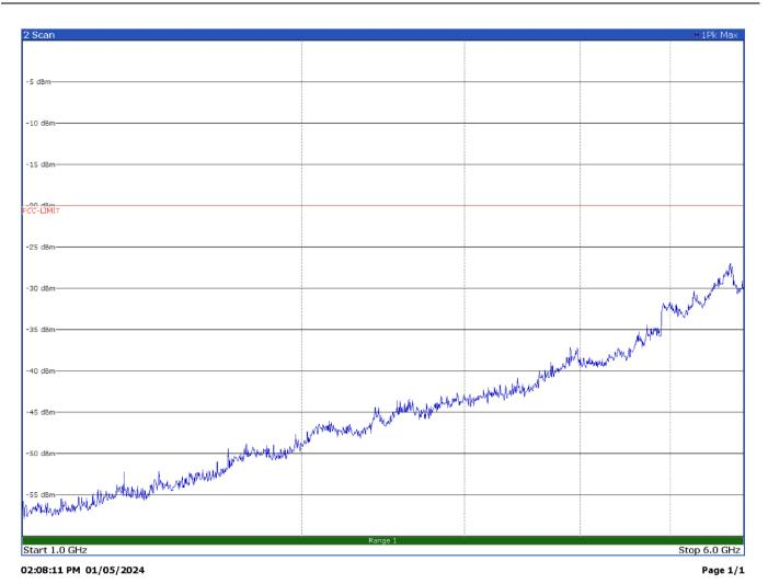
Radiated spurious emissions with modulation DMR 4FSK at 467 MHz – Antenna in horizontal polarization
