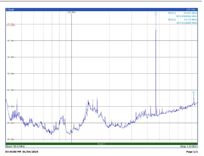
Radiated spurious emissions with modulation FM 12.5 kHz at 467 MHz – Antenna in vertical polarization
