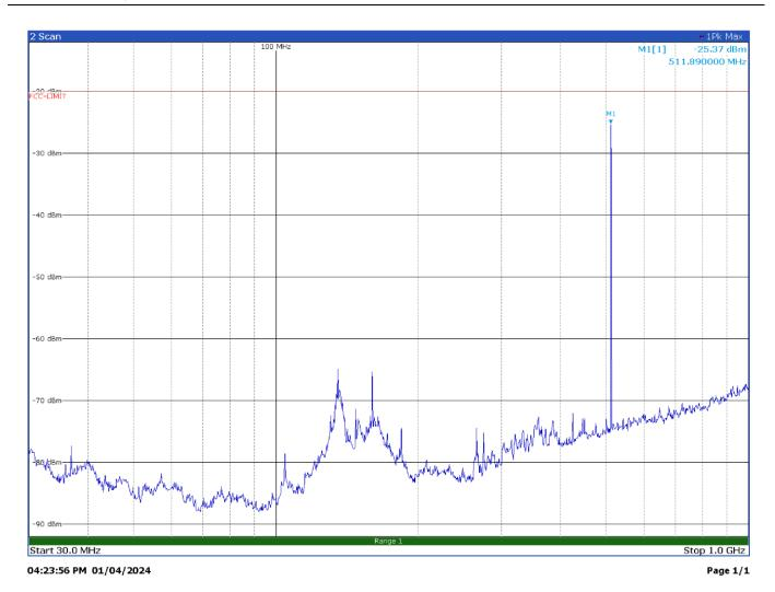
Radiated spurious emissions with modulation FM 25.0 kHz at 511.9 MHz – Antenna in horizontal polarization
