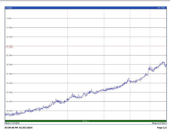
Radiated spurious emissions with modulation FM 12.5 kHz at 467 MHz – Antenna in horizontal polarization
