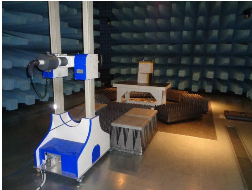
Set-up photo for radiated tests above 1 GHz photo
