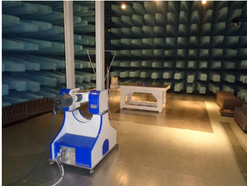
Set-up photo for radiated tests below 1 GHz photo
