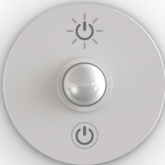
Wireless motion sensor, rolling code 433.92 MHz, recessed with built-in light sensor. CR2450 battery.
