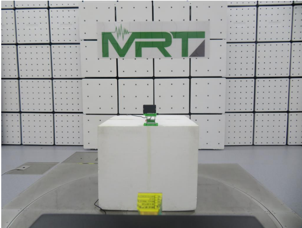
Description: Radiated Emission Test Setup for 140GHz ~ 220GHz
