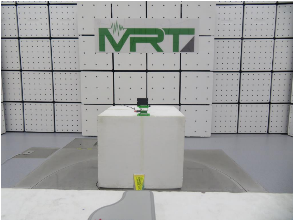
Description: Radiated Emission Test Setup for 75GHz ~ 110GHz
