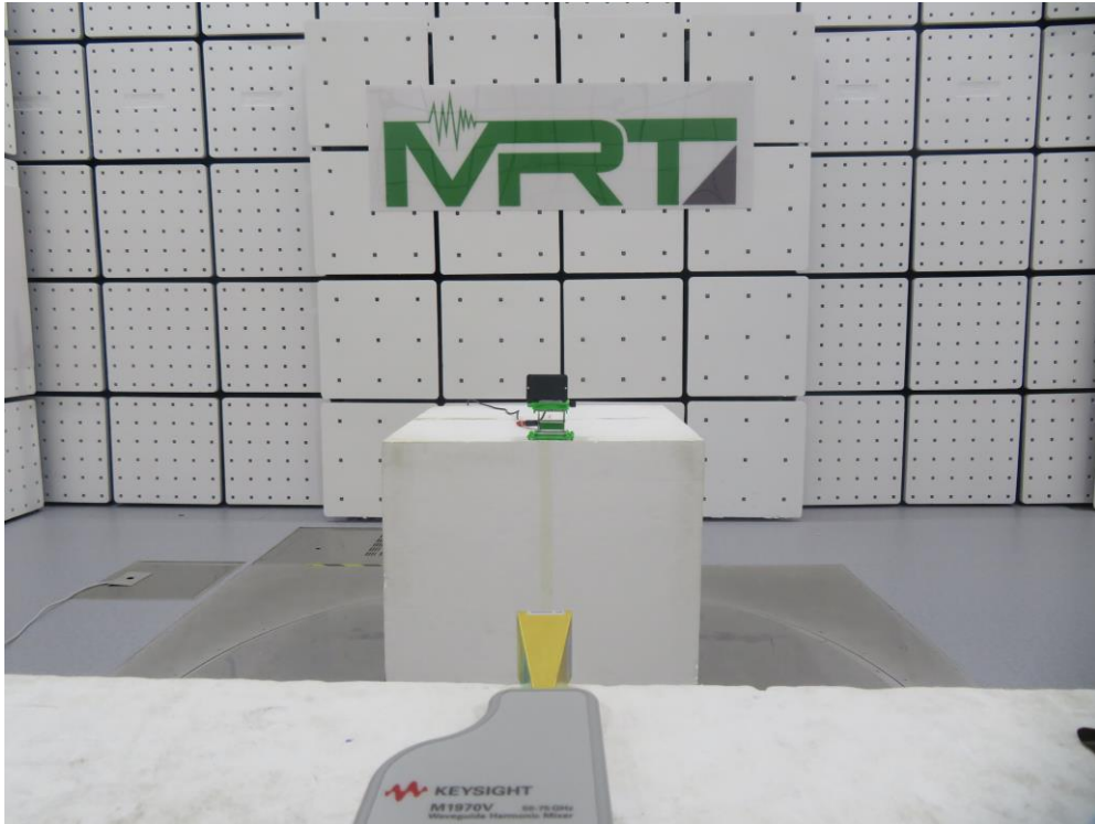
Description: Radiated Emission Test Setup for 75GHz ~ 110GHz
