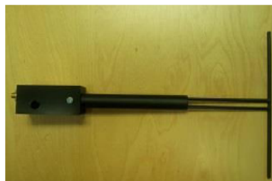
Figure 1 – MVG COMOSAR Validation Dipole
