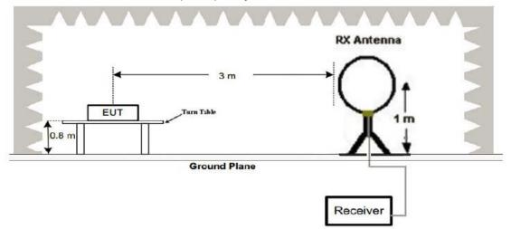
(2) Radiated Emission Test-Up Frequency 30MHz~1GHz
