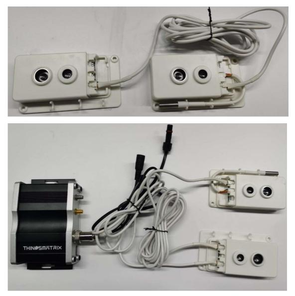
The ultrasonic/temperature cable should go through the drilled hole of the merchandiser and connect to the sensor which need to be fixed on the inner roof of the merchandiser.
