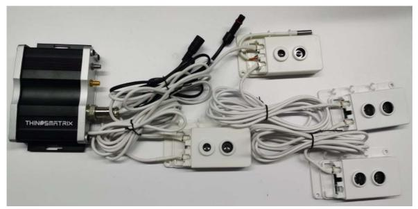
The lidar sensor cable should go through the drilled hole of the merchandiser and connect to the sensor which need to be fixed on the inner roof of the merchandiser.
