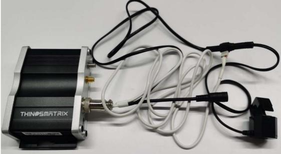
4) Connection the ultrasonic/temperature to the main cable
