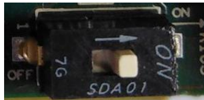
Figure 6 – SBC Switch (SW2)
