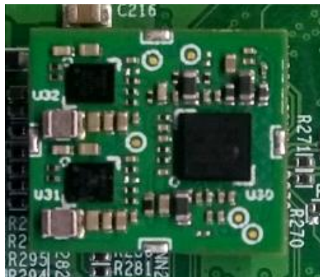
Figure 7 – WCD9335 Audio Code Daughter Board (custom made by elinfochips)
