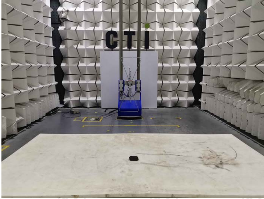
Radiated spurious emission Test Setup-1(Below 1GHz)
