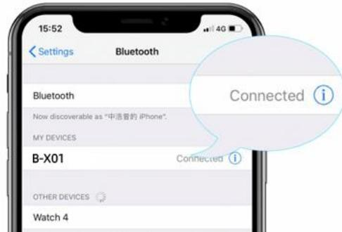
**2. Manual pairing:** Long press the MFB of both earbuds simultaneously for 2 seconds while the both earbuds in power off mode. Keep the distance between the left and right earbud within 10CM, The left and right earbud will be pairing automatically within 10 seconds. Turn on the mobile phone bluetooth and search for the earbuds name, then click the earbuds name for connection, to complete the pairing.
