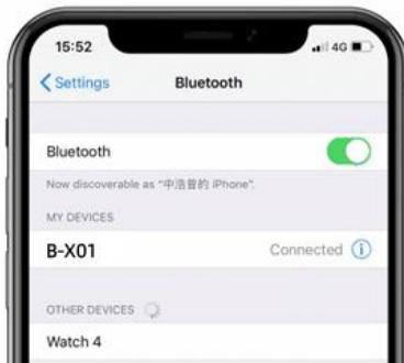
B: Search B-X01 completed, connect to the device well.
