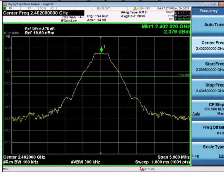
2 Spurious Emissions NVNT ANT1 1-DH5 2402
